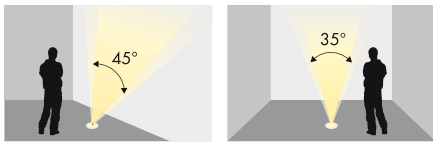
Asymmetrische Linse 45°/35° / Asymmetrical lens 45°/35°
